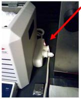
To turn on the spinner, turn the blue air valve behind it counter-clockwise just enough to see the spinner display come on. Do not change any existing recipes. Check the back of logbook for a list of occupied recipes.
