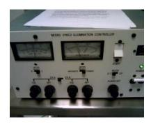
To turn on the mask aligner, turn the power switch to ON position (down).
