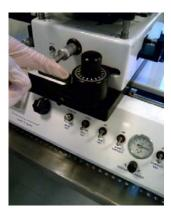
Turning off the mask aligner follows the above steps in reverse: Mask aligner Power switch UP, UV source Power switch UP, turn off vacuum switch on the floor.
