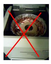
Place aluminum foil if necessary before placing power towel or filter paper and clean the tuck with paper towel wet with acetone. Make sure photoresist does not go through the cylinder holding the tuck otherwise vacuum line will be plugged.
