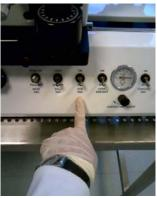
Turn the two level wheels to bring substrate close to the glass photomask. The plastic has been damaged so be <u>very careful</u> when doing this. At the end of the exposure gently place substrate away from the glass photomask if more samples are to be processed. When finished, pull away the substrate stage to a far-away enough distance.
